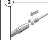
Insert the uberflex hose into trigger handle.
