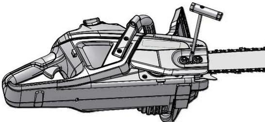
5. When the chain is at the wanted tension, tighten the lock nuts.
