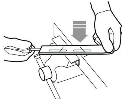
3. Sharpen the top plate, side plate and depth gauge with a flat file.
