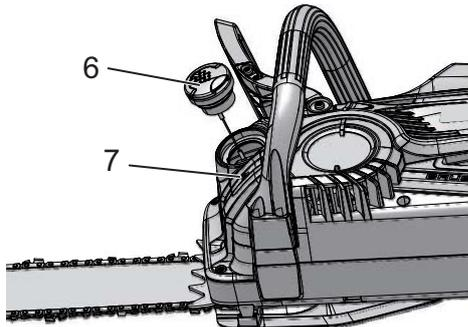
2. Put the oil into the oil tank.
