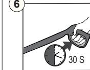
Run water hose for 30 seconds with the motor in OFF position. This helps drain air from the tank and lines.
