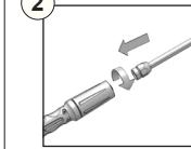
Assemble pressure washer gun to spray wand.
