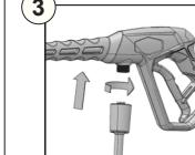
Insert high pressure hose into trigger handle.
