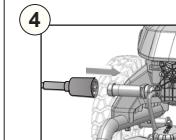
Insert high pressure hose into the pressure washer.
