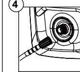
Insert high pressure hose into the pressure washer.
