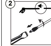
Assemble pressure washer gun to spray wand.
