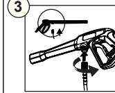
Insert high pressure hose into trigger handle.
