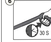
Run water hose for 30 seconds with the motor in OFF position. This helps drain air from the tank and lines.
