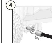
Insert the uberflex hose into the pressure washer.
