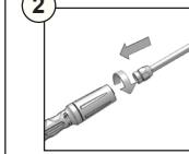
Assemble pressure washer gun to spray wand.
