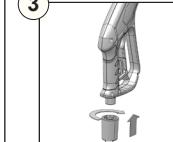
Insert the uberflex hose into trigger handle.
