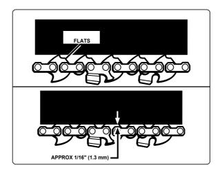
NOTE: A cold chain is correctly tensioned when there is no slack on the underside of the guide bar, the chain is snug, but it can be turned by hand without binding.
